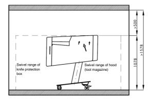
The work area around the machine is at least 0.5 m on all sides; for maintenance work it is at least 1 m; if used as passage way, it is at least 1.2 m.
