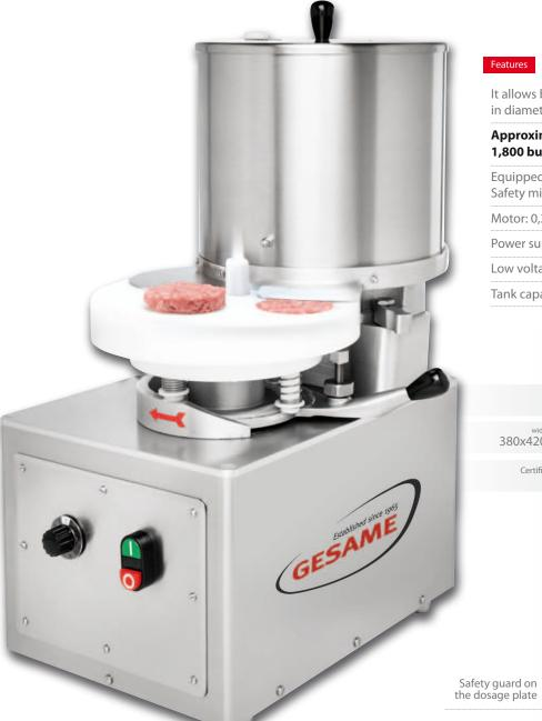
It allows burgers of up to 100 mm in diameter and 25 mm thick.
