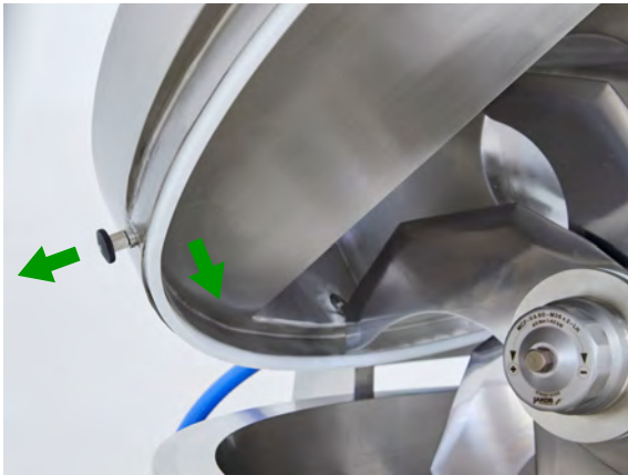
Removeable lid/bowl friction band to facilitate cleaning.
