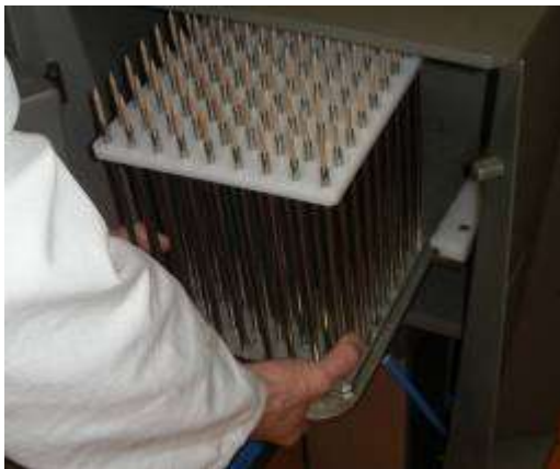
8 INTRODUCE THE SKEWER TUBE ASSEMBLY INTO THE MACHINE CLOSE THE DOOR AND VALIDATE THE CYCLE WITH THE CONTROL LEVER
