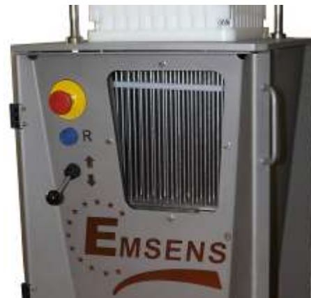
8 INTRODUCE THE SKEWER TUBE ASSEMBLY INTO THE MACHINE CLOSE THE DOOR AND VALIDATE THE CYCLE WITH THE CONTROL LEVER
