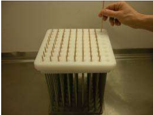
6 INTRODUCTION OF THE WOODEN SKEWERS INTO THE SKEWER TUBE ASSEMBLY THANKS TO A SPECIFIC PLATE
