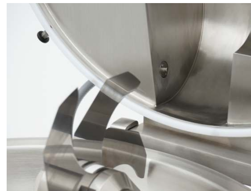
Removable, self-adjusting friction lid/bowl band.
