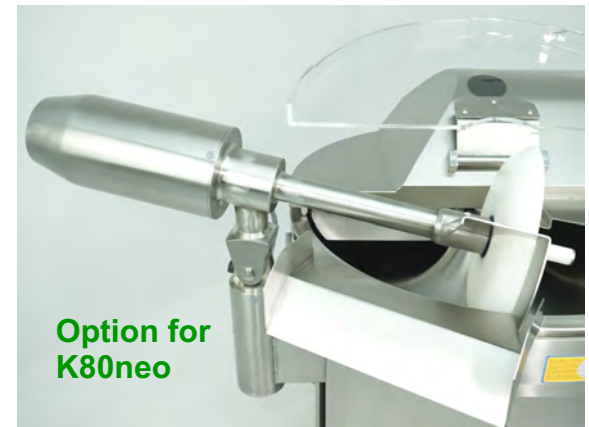
Unloader extracting arm with motorized disc for easy and comfortable unloading.
