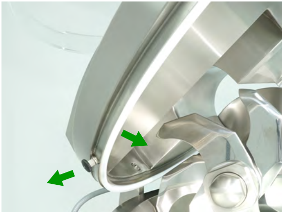
Removeable lid/bowl friction band to facilitate cleaning.
