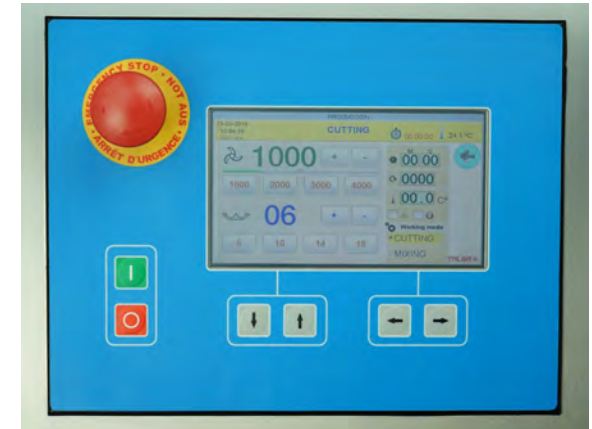
Digital display to control and program all functionalities of the cutter.
