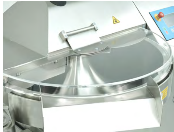
Noise protection cover with automatic decrease of knife speed.
