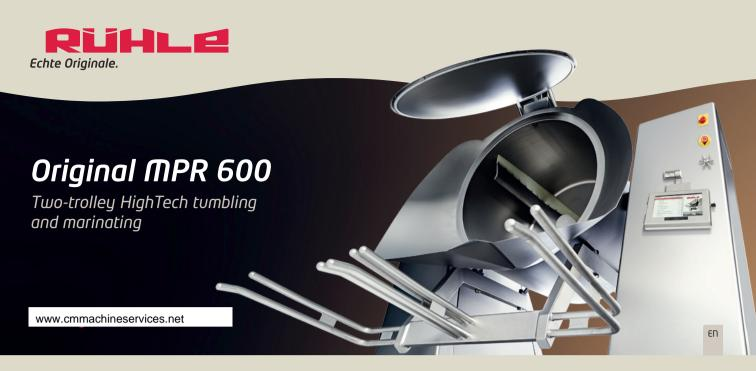
Equipped with a fast feed system, the Original MPR 600 has a container volume of 600 It that can hold 450 kg of meat. From cooling to vacuum treatment to variable arm speeds, it is perfectly equipped to achieve the best possible results. The secret of this successis in its control technology, reflecting decades of experience.
