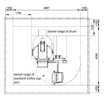
The work area around the machine is at least 0.5 m on all sides; for maintenance work it is at least 1 m; if used as passage way, it is at least 1.2 m.
