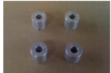
(4) Spacer Stanchions. Used for different Mold Plate thicknesses. May Be Plastic
