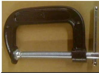
(2) Clamps. Used to secure machine to work table.
