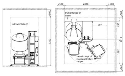
The work area around the machine is at least  $0.5\,\mathrm{m}$  on all sides; for maintenance work it is at least  $1\,\mathrm{m}$ ; if used as passage way, it is at least  $1.2\,\mathrm{m}$ .
