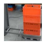
The boxes are pushed onto the fork until they touch the machine.
