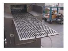
c) Hold the gear rack unit by the connecting bolts and remove the gear rack unit from the guide rollers by lifting it upward. Remove the unit now by pulling it out of the machine on it's feed side.
