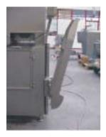
The fork can be swung upward by a 100° when the machine is not in use. This is also the position
