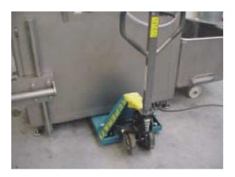
During the **installation and transport of the machine** see to it that the floor can withstand a load of 400 Kg/m². The machine has to be positioned in such a way, that a passable safety path of one meter in width is all around the machine.
