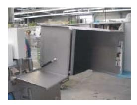
The protective cover is equipped with two shock absorbers which act as a lifting aid covering weights above 20 Kg.
