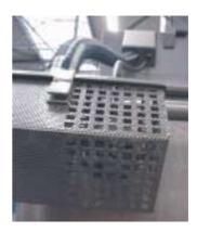
The suction filter always has to be positioned at the base of the brine container in order to avoid the forming of foam on top of the brine. The brine mixing system cuts-off automatically when the brine level sinks below the top edge of the suction filter.
