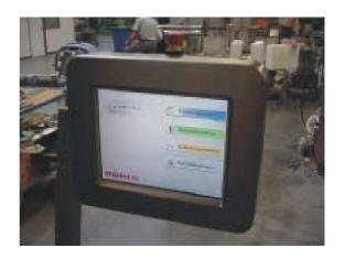
level of the 150 litre container and the 200 litre container respectively. To do this, pull the level sensor out of the machine and position the desired container under it. At the control panel select now the container size and confirm your choice by pressing the key with the green symbol.
