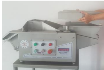
Image 7. Batter belt removal
