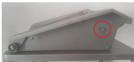
Image 4. Breading belt tensioner
