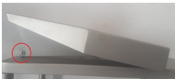
Image 3. Batter belt tensioner
