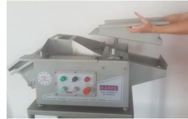
Image 8, Removing batter tank.
