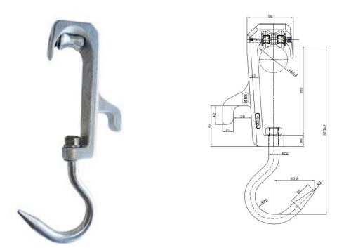
Hook for cattle half-carcases and forequarters transportation Sliding console from flat bar 50 x 12 mm, hot-dip galvanized steel Hook-rod Ø 22 mm, stainless steel 1.4301 Roller and bearing – galvanized steel Up to 1250 kg Weight – 3.82 Length – 410mm
