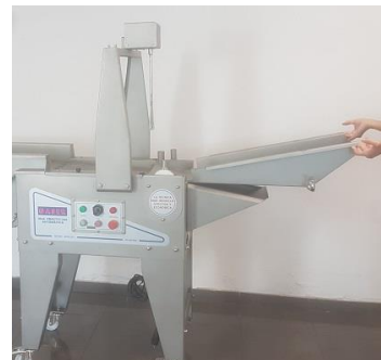
Image 18, Removing batter tank.
