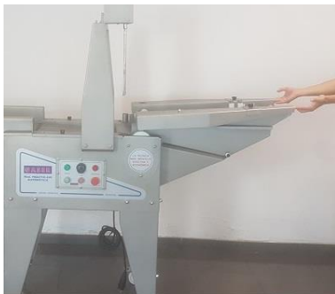
Image 17. Batter belt removal
