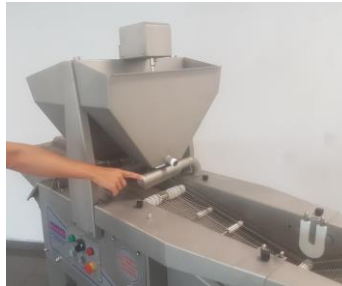
Image 11, disassemble elbow and outlet mouth of blower
