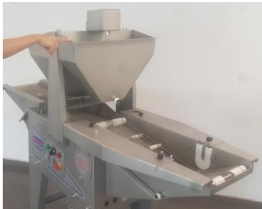
Image 12, Removing batter tank
