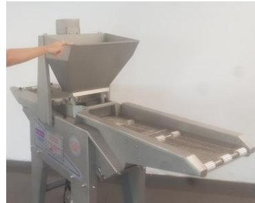
Image 13, Removing bread tank
