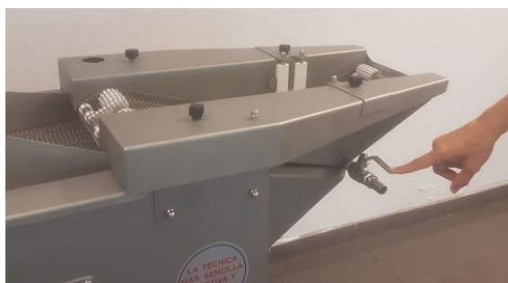
Image 9. Emptying batter tank
