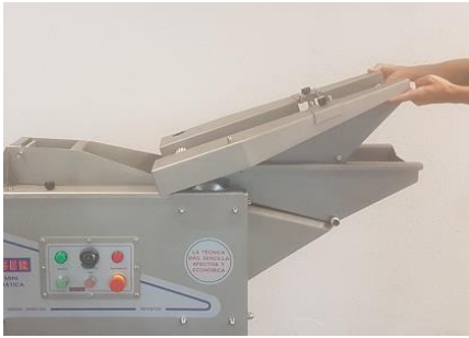
Image 11. Batter belt removal
