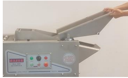
Image 12. Removing batter tank
