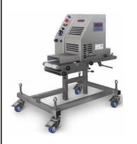
This setup is to work with Grinders or Mixer Grinder. The stand or table is included with the machine and is adjustable with minimum height of 527mm and maximum 764 mm.
