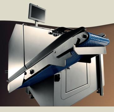
This semi-automatic machine has a high cutting rate and produces up to 3,000 kg of cubes, strips or portions per hour. This performance is due to the large shaft and fast operating speed as well as (and especially) to time-saving features that prevent idle cuts.
