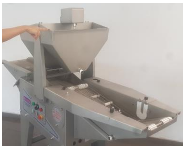
Image 9, Removing batter tank
