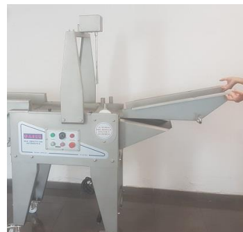
image 15, Removing batter tank.
