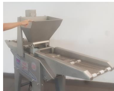
Image 10, Removing bread tank
