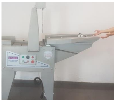
image 14. Batter belt removal
