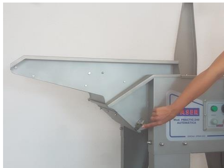
Image 16. Opening the discharge door
