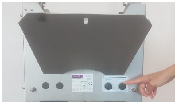
Image 17. Use direction reverser
