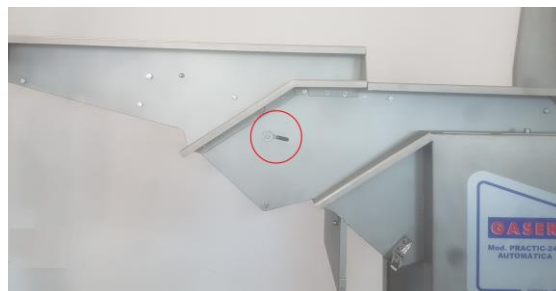
image 6. Breading belt tensioner
